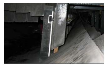
IMTECH®'S "belt-friendly" rubber liners can nearly touch the conveyor belt, forming a tighter seal without damaging the belt.
